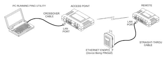
To conduct a PING test, an Ethernet-enabled device must be connected to the Remote, and it must have a compatible IP address. Remote radios do not have a reladeress and cannot be verified directly using this method.
